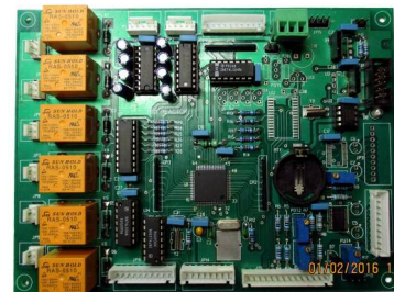
ATMEL AVR ATMEGA128 RISC microcontroller based single board computer
