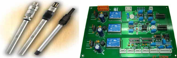
Three stage galvanic & two stage optical isolation signal conditioner
