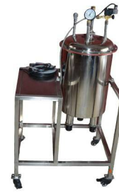
S.I.P system for i-situ sterilization (optional accessory)
